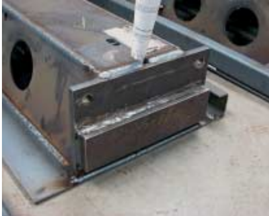
Fig. 2 One of the customized options on offer is the production of a composite beam accommodating varying slab heights – the perfect solution whenever two floor bays with considerable differences in length are located next to each other.
